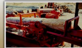
The all steel infeed conveyor is fabricated from 5/8" formed plate steel with 3/8" gussets is equipped with Morbark's exclusive all-steel welded track type chain
