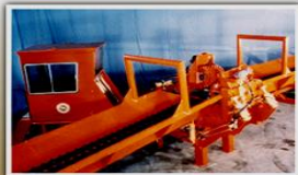
The trough-type infeed and outfeed conveyors are variable in length up to 80'.
